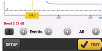
Bend as seen on an OTDR trace
