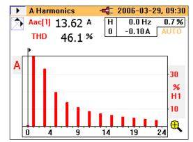
Figure 6. Current harmonics bar graph.
