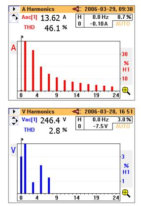
Figure 2. Graph harmonics for voltage and current.
