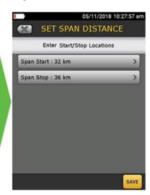
Process to set Span on an OptiFiber Pro OTDR
