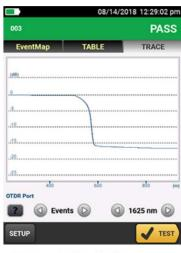
Splitter as seen on an OTDR trace
