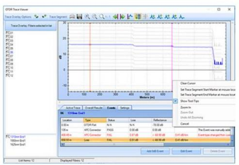
Setting span event parameters using LinkWare PC
