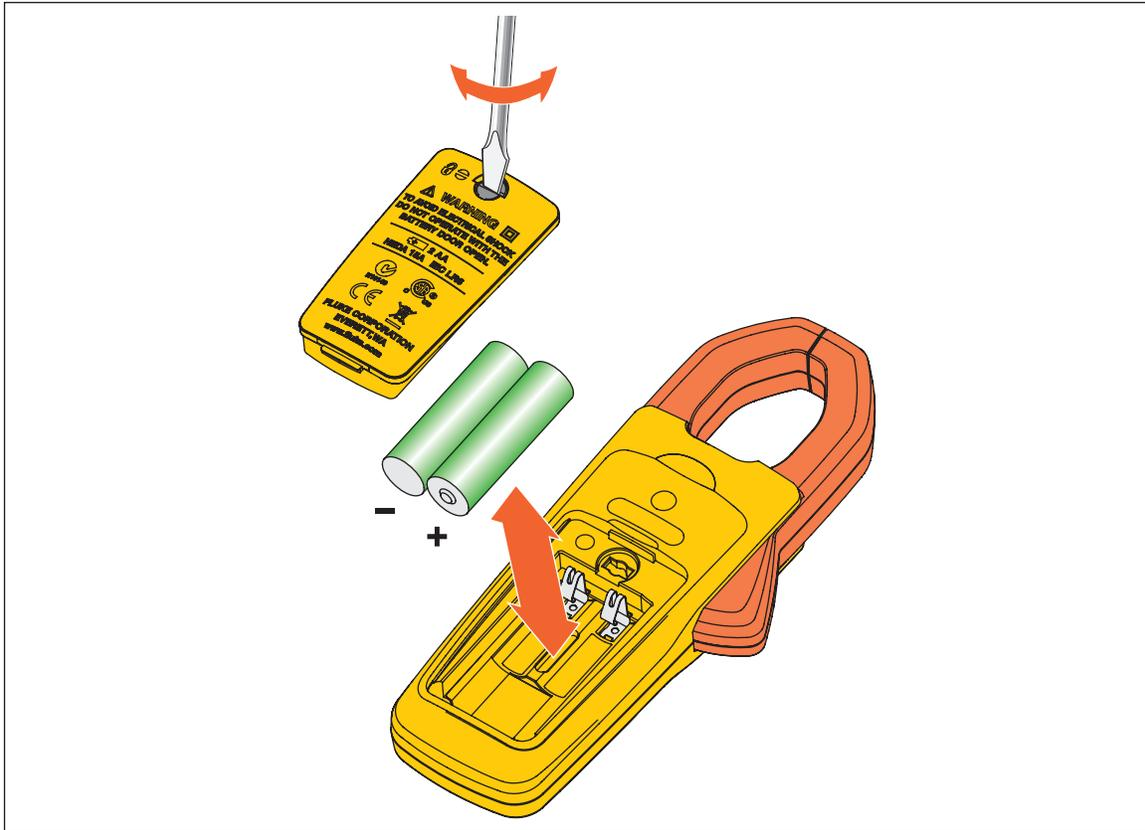
Figure 5. Battery Replacement
