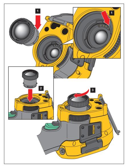
Figure 1. Optional Lens Installation
