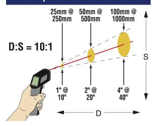
The MiniTemp MT6 thermometer is intended for close range targets, measuring a minimum target area of 1 inch in diameter from a distance of approximately 10 inches, and measuring approximately a 6 inch area from 5 feet away.
