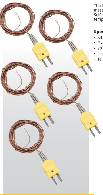
This K-Type thermocouple is designed for temperature measuring applications and is compatible with Fluke Solmetric SolSensor. The thermocouple can be used to measure temperature range from 0 °C to 482 °C (32 °F to 900 °F).
