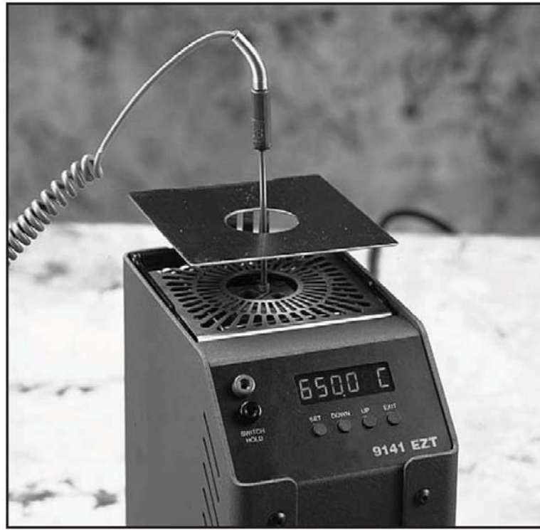
Figure 1 Heat shield installed on 9141 calibrator
