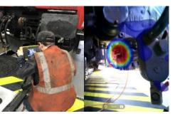
To ensure safety on the tracks, the maintenance technicians pay special attention to the braking system. The centralized pneumatic brake system is used to keep pressure on the system continuously and to ensure the brake shoes remain open. As soon as the pressure drops, the brakes engage and start causing undesired friction on the axles. A tricky, tiny leak in the compressed air system can lead to system malfunctions, which activate the brakes. These errors must be corrected as soon as possible.
