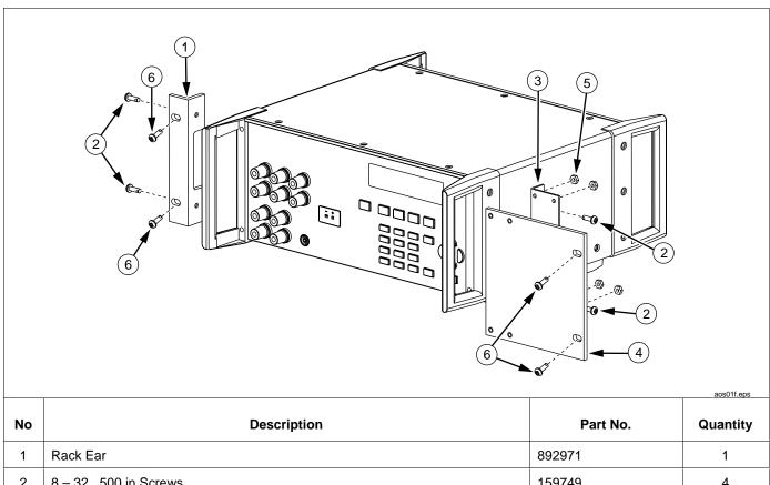
8 - 32, .500 in Screws Rack Panel Bracket Rack Panel Filler Plate 6 - 32 Nuts 10 - 32, .750 in Screws 525A Rack Mount Kit Instruction Sheet (this document - not shown)
