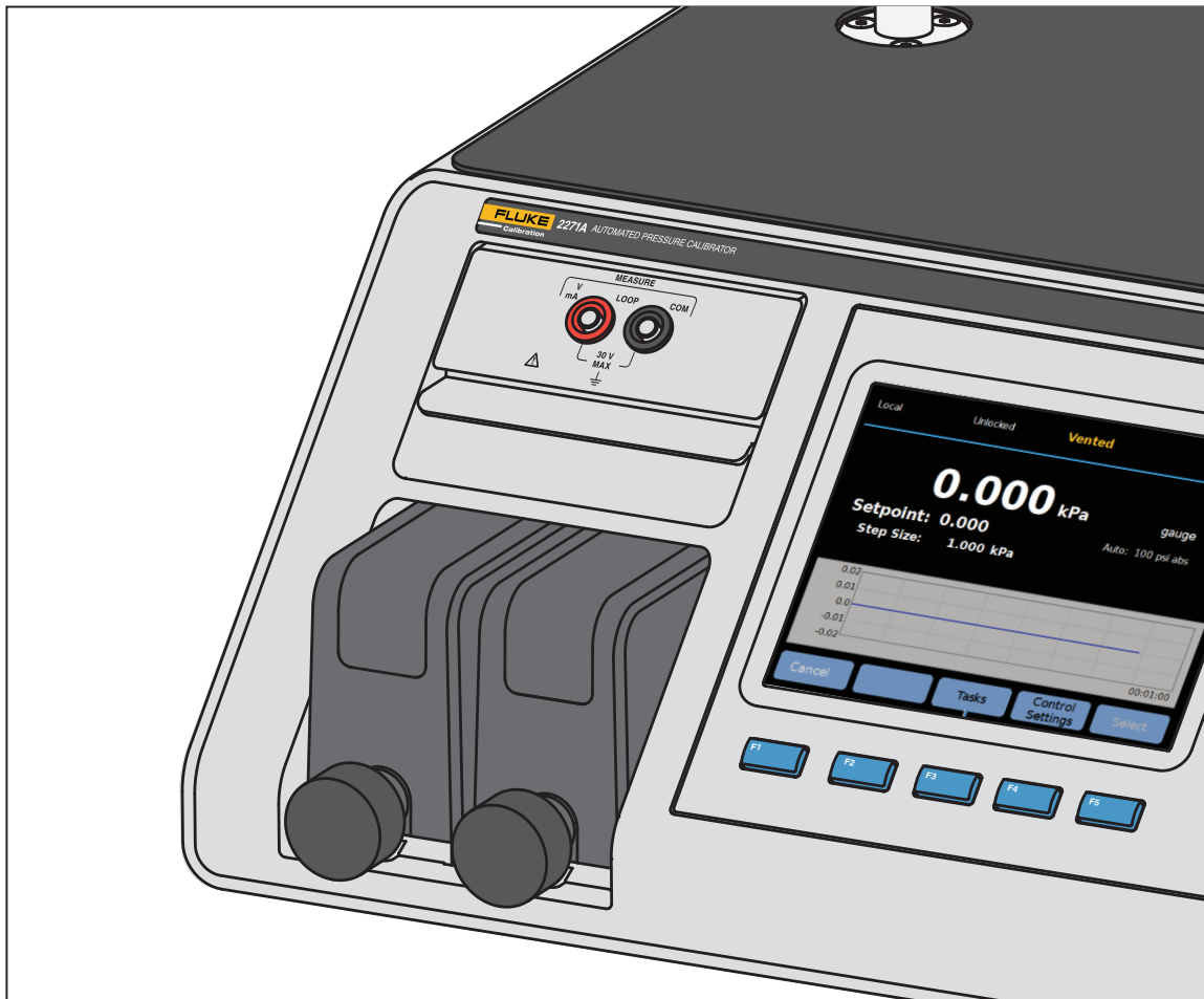
Figure 3. Installed EMM and PMM Modules
