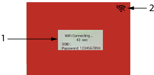
Figure 12.2 Wi-Fi Connecting Screen
