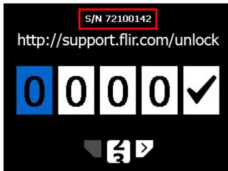
6. To complete the registration and unlock the camera, you must enter an unlock code into the camera. The code is available in your FLIR account, under *My Products*.
