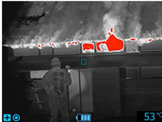
Figure 12.7 Heat detection mode.
