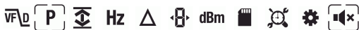
Figure 5.3 Mode icons (AC voltage measurements): Peak mode and Silent mode are enabled
