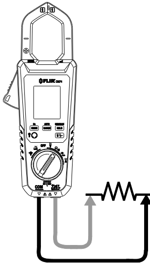
Figure 5.5 Resistance and Continuity Measurements
