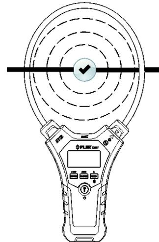
Positioning Conductor in Center of Clamp Jaw
