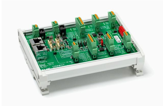
**Figure 12.1** A-series connection board
