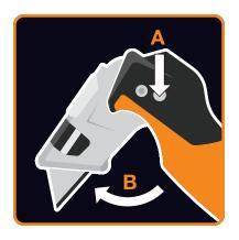
Press the button on the side of the knife (A) to flip knife to open position (B).
