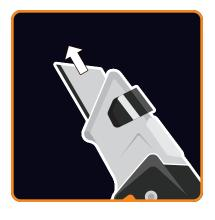
3. Pull the blade out of the front of the knife.
