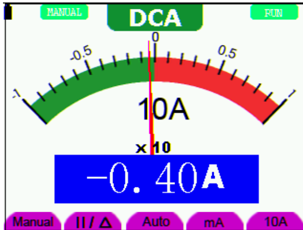
Figure 9: 10A DC Current Measurement
