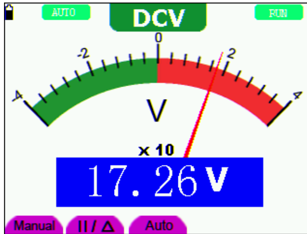
Figure 6: DC Voltage Measurement
