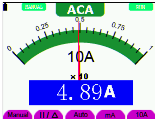
Figure 11: AC Current Measurement for 10A
