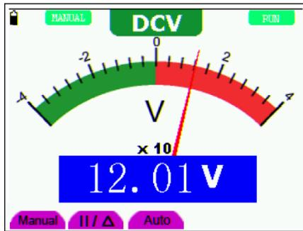
Figure 13: Automatic/Manual Range Adjustment
