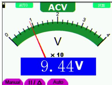
Figure 7: AC Voltage Measurement
