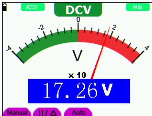
Figure 6: DC Voltage Measurement
