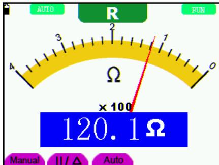
Figure 2: Resistance Measurement
