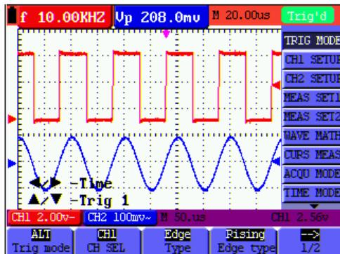
7. Press ◀ (yellow) or ▶ (yellow) to adjust the time base horizontal position and press ▲ (yellow) or ▼ (yellow) to adjust the trigger horizontal position for Channel 2.
