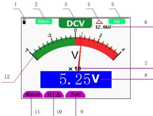
Figure 1: Multimeter Display Window
