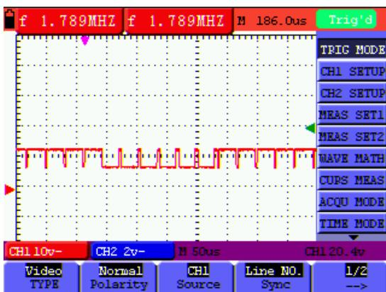
Fig. 25: Video Line trigger (screen 1)
