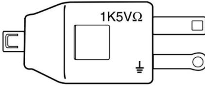
Fig 40: 5V square wave output adaptor
