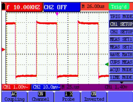
Figure 17: Inverted Waveform
