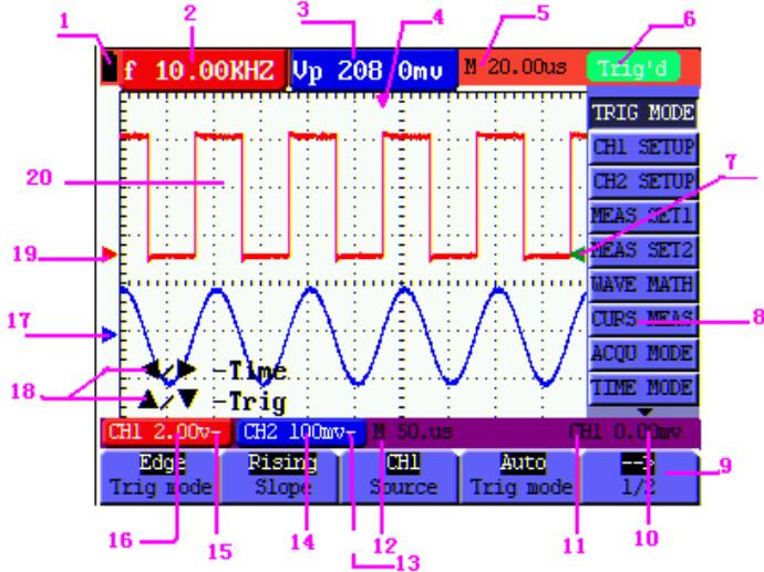
Figure 4: Oscilloscope Display Screen
