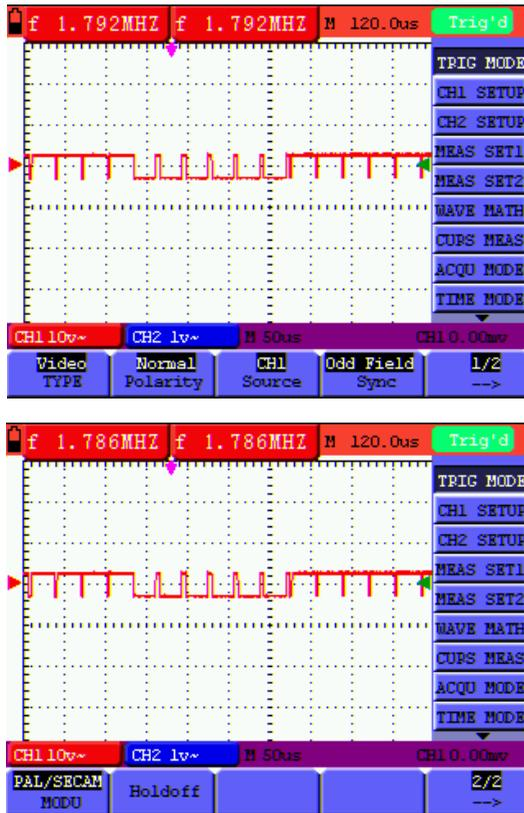
Figure 24a (screen 1) and 24b (screen 2): Odd Field Video Trigger
