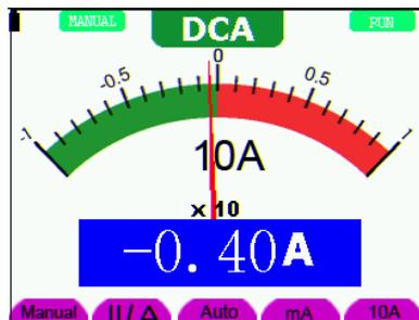
Figure 9: 10A DC Current Measurement
