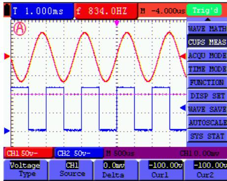
Figure 36-a: Use the Cursor for a Voltage Measurement
