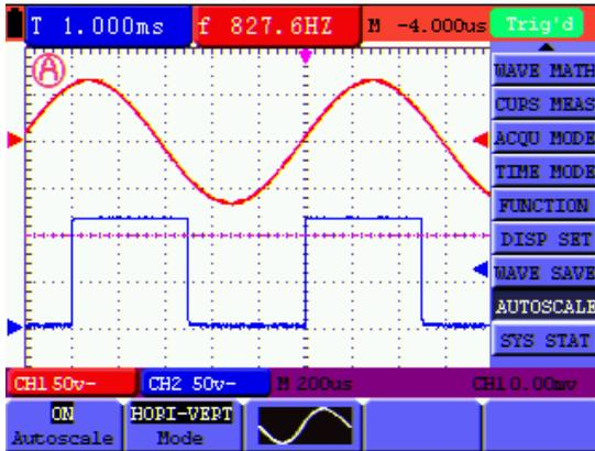
Fig 33: Autoscale Horizontal - Vertical mono-period waveform
