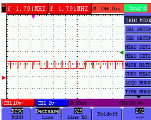
Fig. 26: Video Line Trigger (screen 2)
