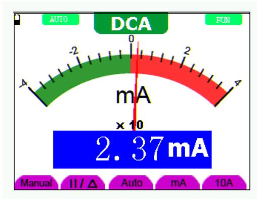
Figure 8: 400mA DC Current Measurement
