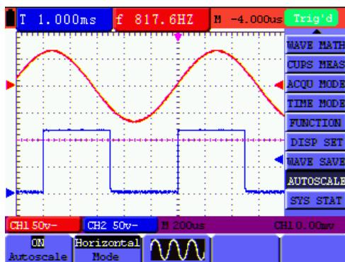
Fig 35: Horizontal mode multi-period waveform
