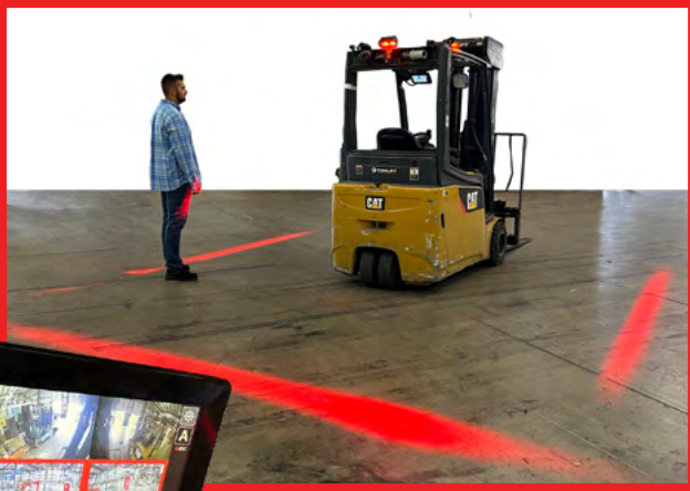
In cab display highlights pedestrian
