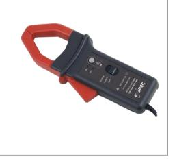
Elspec's current clamp (SOA-0270-1400) measures DC or AC currents, without opening the circuits they are flowing in. The current clamp is used as an accessory for the G4500 BLACKBOX Portable. This clamp measures DC current up to 1500 A and AC current up to 1000A. It outputs the form and amplitude of the current measured as a voltage image of the primary curre nt.
