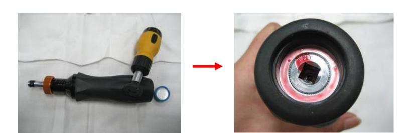
Use Nut Screwdriver/hand to remove end cap from handle base.
