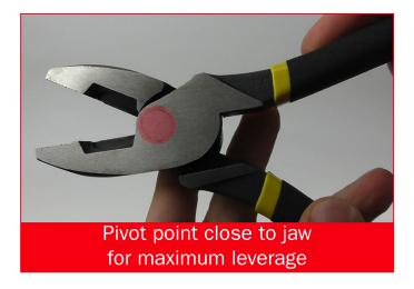
Heavy Duty Lineman's Pliers are used to cut, straighten and bend wire as well as to twist wires together when making splices. Made from high-quality carbon steel with a hardened finish for durability, these pliers' tapered head allows for easy work in tight spaces, and provides a self-opening action which supplies smooth operation.
