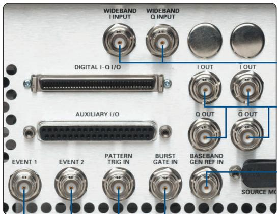
1 GHz RF modulation BW I/Q inputs
