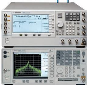
Setup for utilizing Signal Studio software for pulse building to apply pre-distortion to calculated waveforms for improved image rejection and RF flatness.
