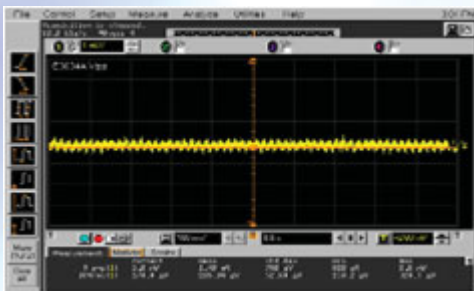
Agilent E3634A - V_{\text{pp}} mean = 1.49mV
