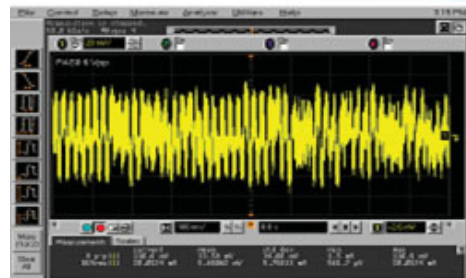
Other power supply - V_{\text{pp}} mean = 33.59mV
