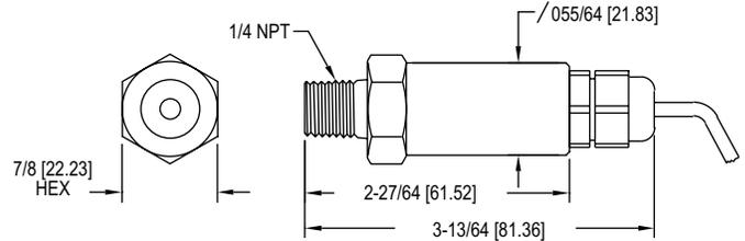
The **Series 626 & 628 Pressure Transmitters** converts a single positive pressure into a standard 4-20 mA output signal. The Series 626 and 628 can be used to accurately measure compatible gases and liquids; Series 626 full-scale accuracy is 0.25%; Series 628 full-scale accuracy is 1.0% (see specifications). Designed for industrial environments with a NEMA 4X (IP66) housing, this transmitter resists most effects of shock and vibration.
