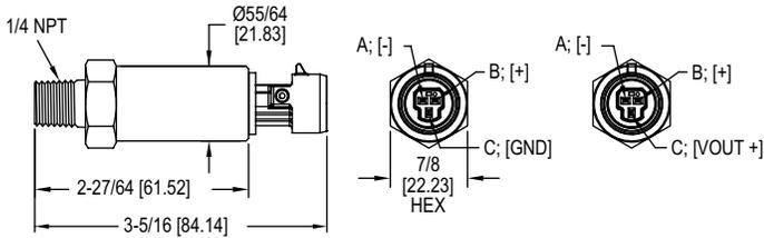
Figure D: Packard Connection
