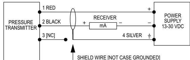
Figure A: Current output connection
