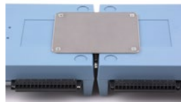
Figure 3. USB-2416-4AO secured to an AI-EXP32
