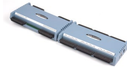
Figure 2. USB-2416-4AO directly connected to an AI-EXP32
