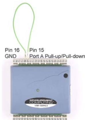
Figure 3-6. Pull-down connection for Port A
