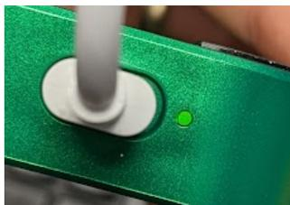
Figure 9. A dim LED when only the digital rails are enabled but the device is not active.
