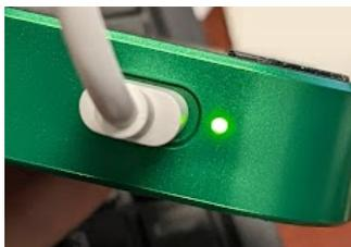
Figure 8. A fully bright LED when the digital and analog rails are active.
