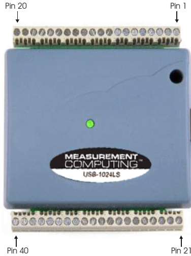
Figure 3-2. USB-1024LS screw terminal pin numbers
