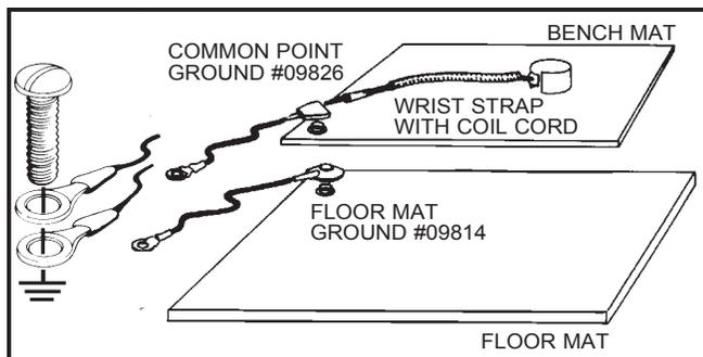
Figure 1. Common point ground for each workstation
