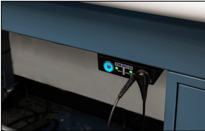
Figure 9. Using the ParkSnap™ on the Multi-Mount Continuous Monitor to store a wrist cord
