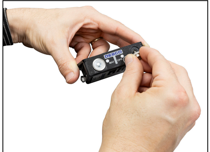
Figure 7. Installing the 10 mm ParkSnap™ to the 19337 Multi-Mount Continuous Monitor
