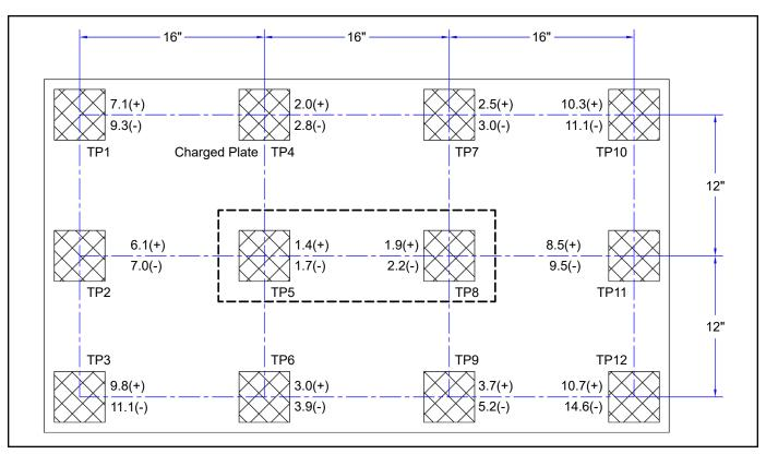
Figure 15. 60640, 60467 Neutralization (Discharge) Times at 120VAC, 60Hz input
