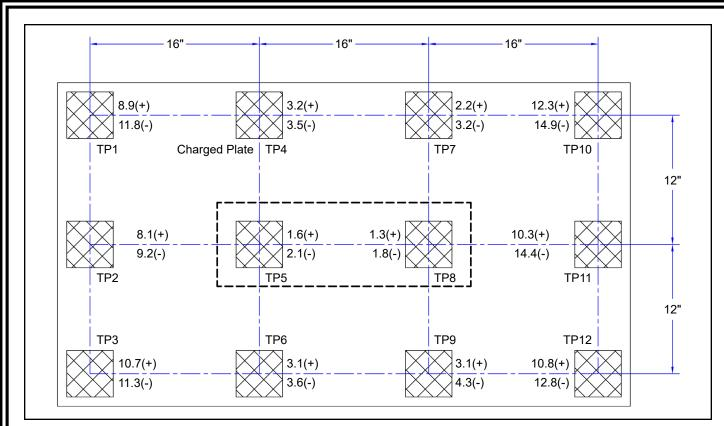
Figure 16. 60640, 60467 Neutralization (Discharge) Times at 220VAC, 50Hz input
