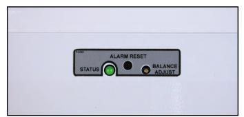
Figure 9. Calibration controls
