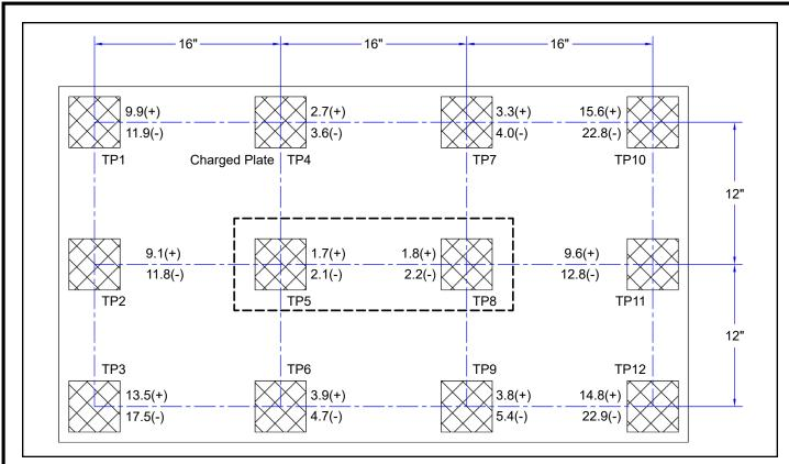
Figure 14. 60640, 60467 Neutralization (Discharge) Times at 100VAC, 50Hz input
