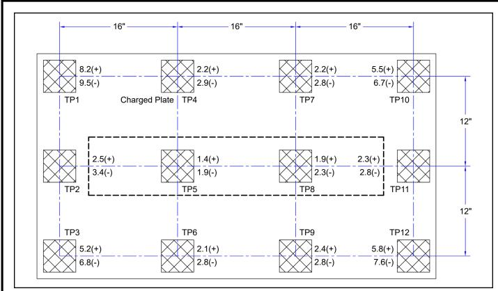
Figure 12. 60473, 60468 Neutralization (Discharge) Times at 120VAC, 60Hz input
