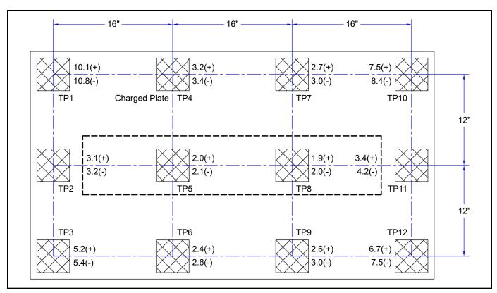
Figure 13. 60473, 60468 Neutralization (Discharge) Times at 220VAC, 50Hz input
