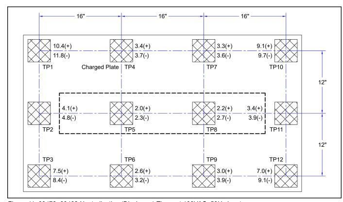
Figure 11. 60473, 60468 Neutralization (Discharge) Times at 100VAC, 50Hz input
