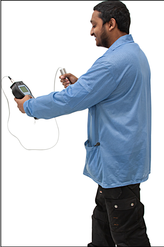
Figure 5. Using the Body Voltage Monitor
