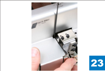
23 Tighten the rail fixing screw in clockwise direction
