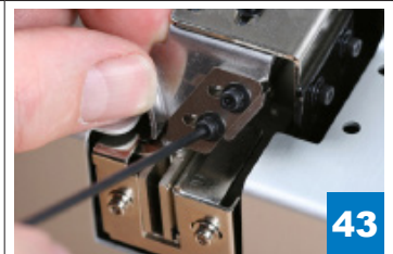
43 Slightly loosen screws shown
