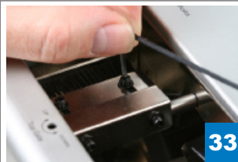
33 Slightly loosen screws shown in counter-clockwise direction
