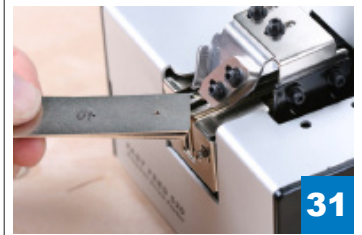
31 Remove measurement shims
