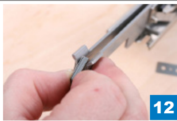
12 Insert the spacer shims into rail assembly
