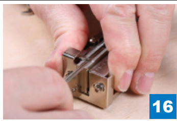
16 With the previous screws loosened, squeeze the rail sides until the rails bottom against the measurement shims
