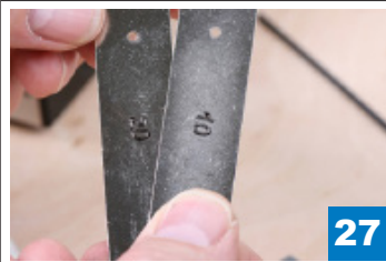
27 Choose the correct combination of measurement shims according to the fastener head height +0.5 mm
