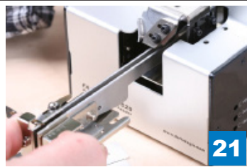
21 Guide rail assembly into the feeder
