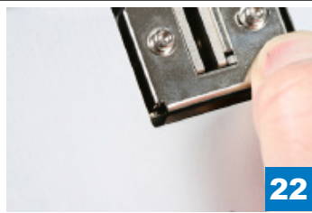
22 ...and push until rail stops Note - the bent angle of the rail assembly slides under the sensor plate
