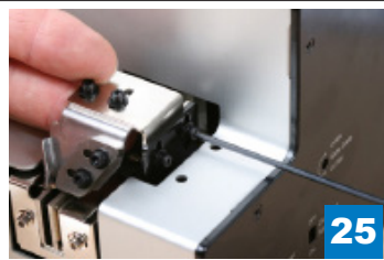
25 Slightly loosen screws shown in counter-clockwise direction
