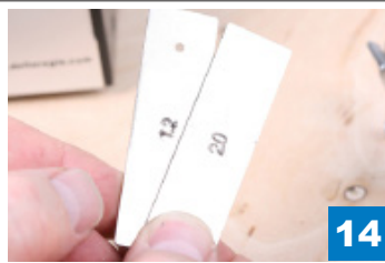
14 Choose correct combination measurement shims according to screw diameter +0.2 mm
