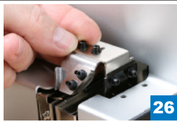
26 Bit guide can now move freely up and down
