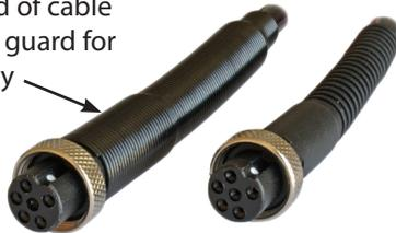
Push cable connector firmly into receptacle and secure retaining nut hand-tight. Do not overtighten.
