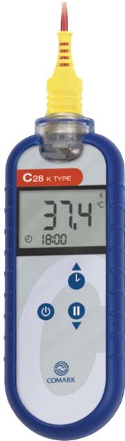
This Type K thermocouple thermometer has an easy-to-use keypad and a large, clear LCD display with a permanent clock. A cell-phone style menu allows the auto switch-off to be changed to 3, 10 or 30 minutes and the countdown timer to be set – the timer can also be stopped during countdown. The case incorporates a built-in protective boot and is waterproof to IP67 standard.
