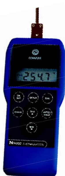
Compatible with 8 thermocouple types – K, N, T, J, R, S, E and B. Twin sub-miniature probe connectors allow differential temperatures to be measured, with readings displayed in °C, °F or K. It can also be used as a conventional thermometer when a single probe is connected.
