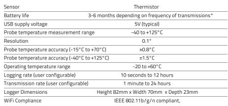
supports WEP, WPA/WPA2 encryption and enterprise networks (PEAP, EAP-FAST, EAP-TTLS)
