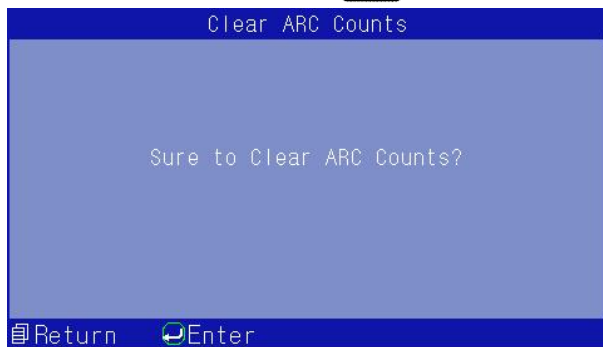
Fig.B-5 Confirmation menu of ARC counts clear-up
