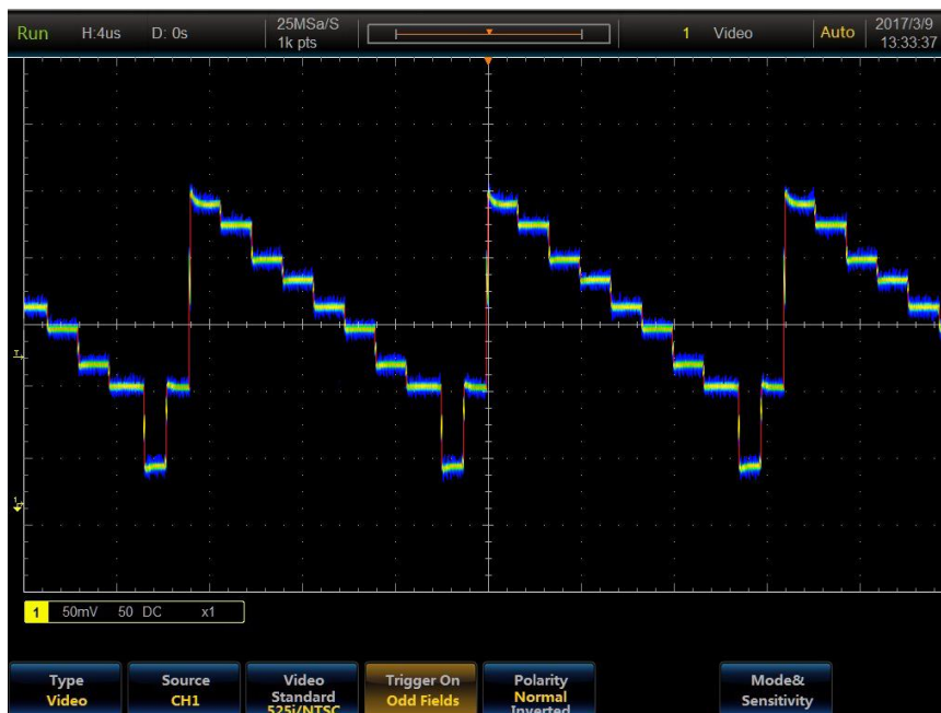
Fig. 5.40 Video Trigger Example
