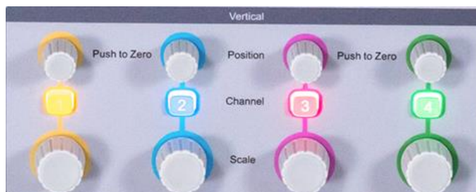
Fig. 2.15 Vertical System Setup Area
