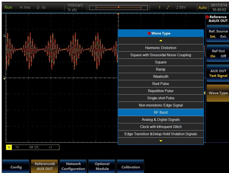
Fig. 5.51 RF Test Signal Example
