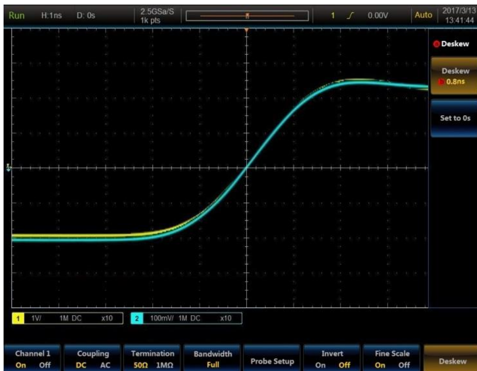
Fig. 3.14 Deskew Calibration Example
