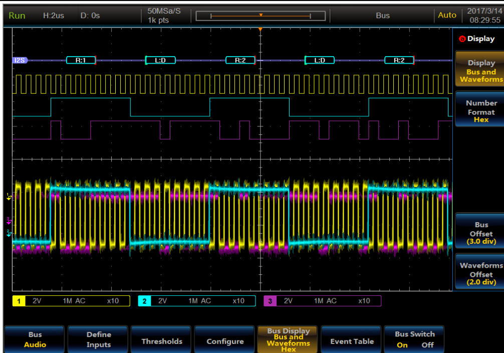
Fig. 11.191 Audio Trigger and Analysis Example
