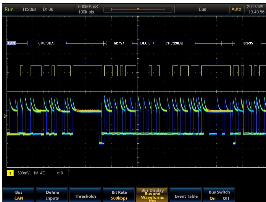
Fig. 11.99 CAN Trigger and Analysis Example
