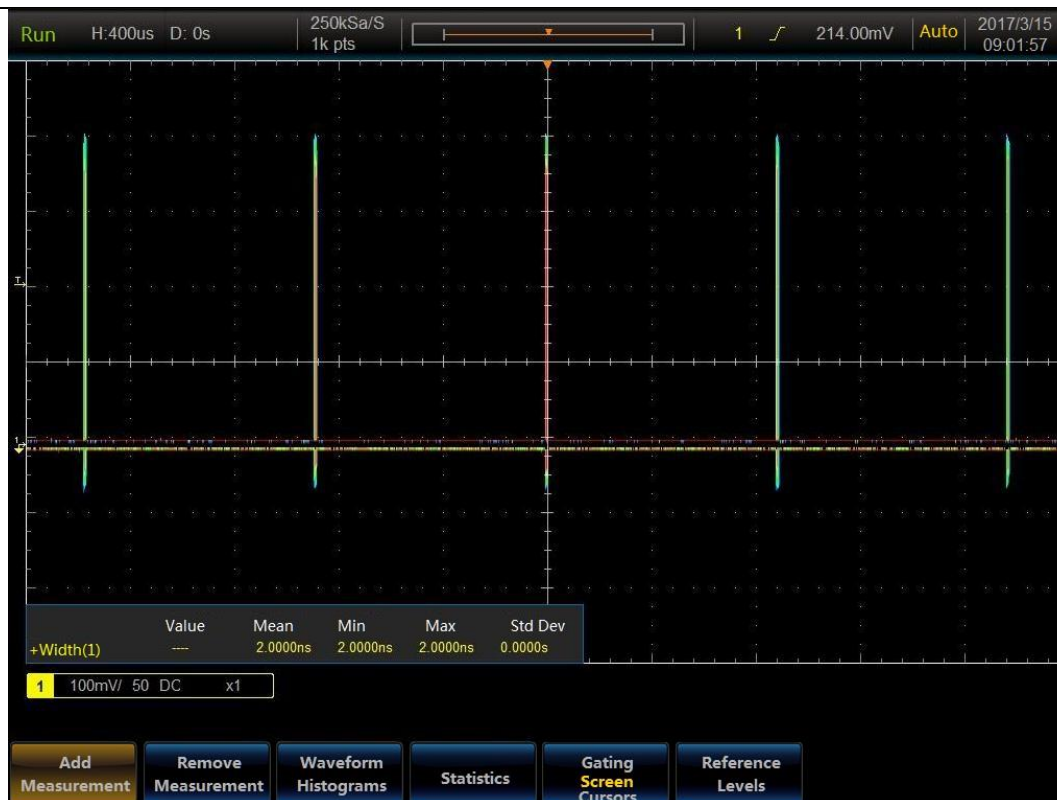
Fig. 19.2 Example of Pulse Measurement by Using Peak Detect Mode
