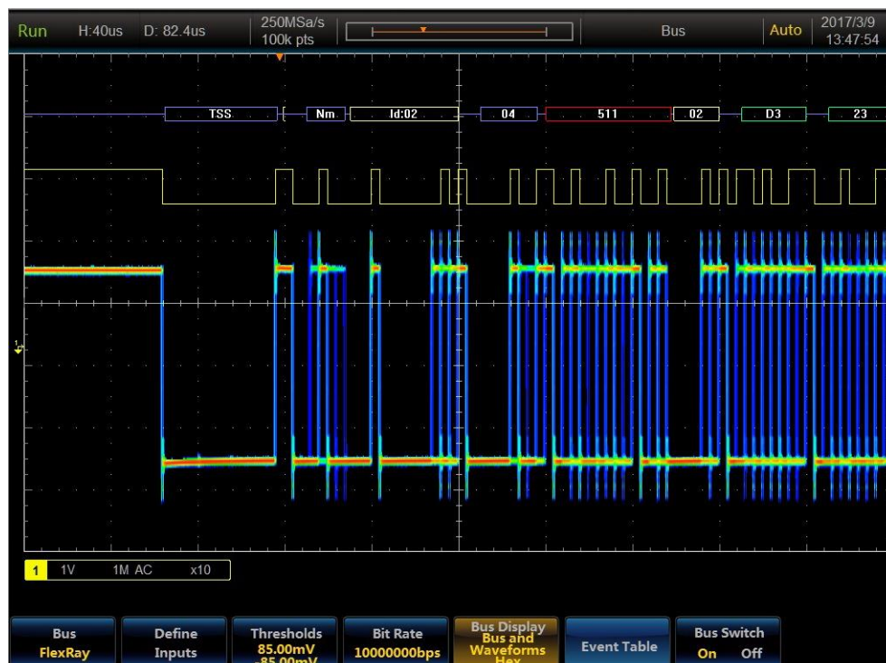
Fig. 11.165 FlexRay Trigger and Analysis Example
