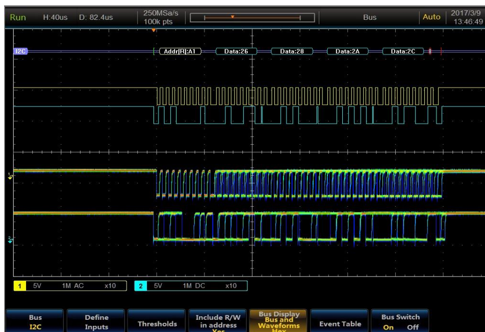
Fig. 11.27 I2C Trigger and Analysis Example
