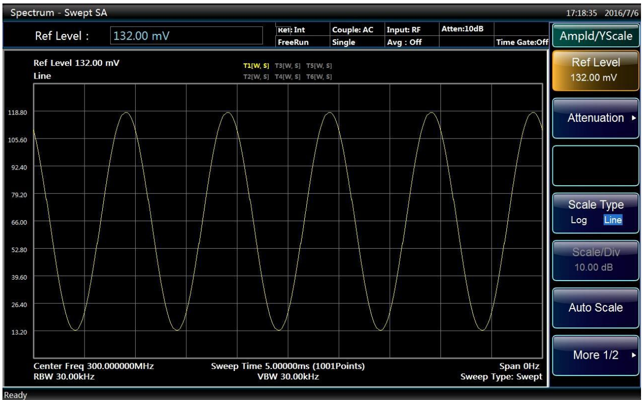
Fig. 4.36 Measure AM signal modulation depth with demodulation waveform
