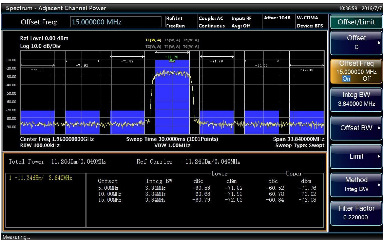
Fig.4.67 Measuring third adjacent channel
