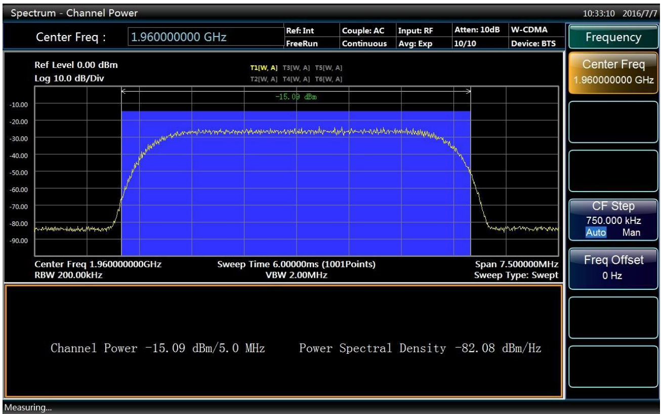
Fig 4.62 Results of channel power measurement
