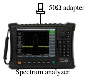
Fig. 12-8 Setting for Display Average Noise Level Test
