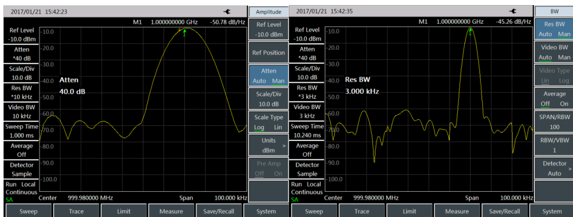
Fig. 4-11 Noise Measurement by Noise Marker Function
