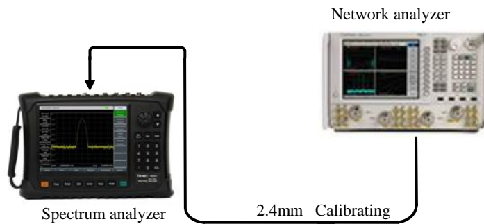
Fig. 12-18 Voltage Standing Wave Ratio Test of Input Port
