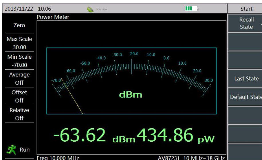
Figure 4-1 Power Test Interface
