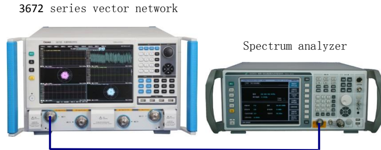
Fig. 11.3 Block Diagram of Test of Harmonic/Non-harmonic Suppression Test
