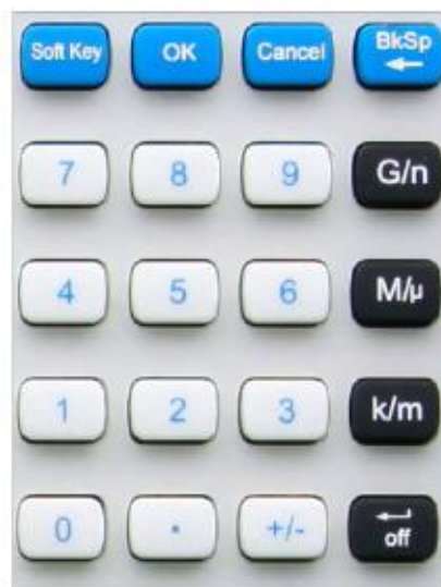
Fig. 3.19 Input Key Zone of 3672
