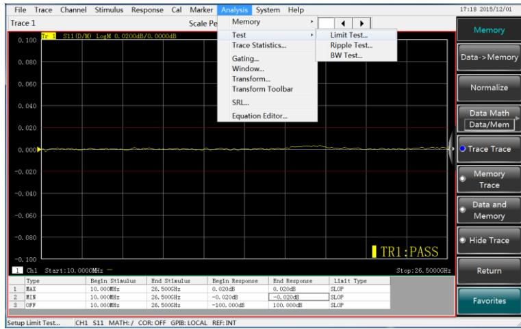
Parameters can be quickly input through activated input toolbar. It can improve the test efficiency to setup the limit line and segment sweep value for production line.
