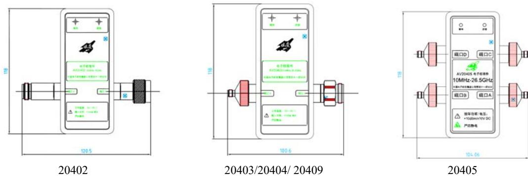
Note 1: The height of the above 2040X series electronic calibration modules are all 50mm.
