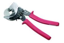
Ratchet Cable Cutter, Cuts up to 336 kcmil ACSR, 500 kcmil AL, 350 kcmil CU.
