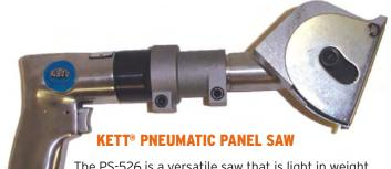
The PS-526 is a versatile saw that is light in weight and portable, making it perfect for use in the aircraft maintenance industry. Cuts mild steel up to 16 gauge or aluminum up to .250". Uses metal 1-3/4" or 2" diameter metal blades with a 7/16" arbor hole. Depth of cut is easily adjustable with use of the panel guard. Manufactured by KETT Tools, considered the leader in pneumatic saws. 11" long, weighs 4 lbs. Includes four blades to get you started - replacement blades are readily available.
