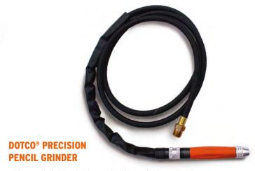
This small, lightweight pencil grinder features a .1 horse power motor and is perfectly balanced for precision use. Industry standard 1/8" collet. Operates at 60,000 rpm. Rear exhaust. 5.8" long, weighs only .3 lbs! **Made in the USA!**
