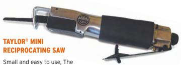
T-7702 cuts straight or curved patterns. Can cut aluminum, mild steel, plastic and fiberglass with ease. Comes with two blades (24 & 32 TPI), extra blades are available. Operates at 10,000 strokes per minute. Weighs 1-3/8 lbs, 7-1/8" long. Depth of cut is adjustable with use of built in guard. High quality import.
