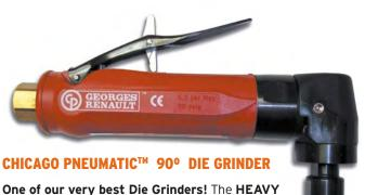
One of our very best Die Grinders! The HEAVY DUTY gears in the head of this tool are unlike any other tool on the market and are specifically designed to hold up under the toughest conditions. Full 1/2 horse power motor spins at 20,000 RPM and offers the power needed to handle the most difficult jobs. 1/4" Collet is standard. Weighs 1.13 lbs, 6-1/2" long. This is a top of the line Die Grinder, that will provide years of dependable use. Collet wrenches included.
