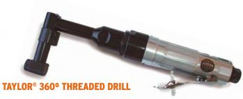
Great for getting into tough areas! The angle head can be rotated and locked a full 360°. Housing is milled from solid stock. Grease fittings in head and body permit you to easily lubricate the tool and prolong gear life. Uses industry standard 1/4-28 threaded drill bits. 2800 rpm, 10.8" long, weighs just 1.98 lbs. High quality import.
