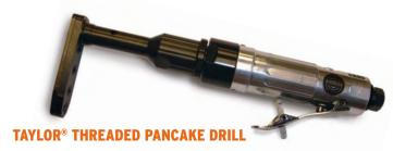
Another great threaded drill designed to access tough areas. Uses industry standard 1/4-28 threaded drill bits. "Pancake" head is 3" long, 3/8" thick, and 7/8" wide. 2800 rpm. 10.25" long, weighs 1.9 lbs. High quality import.
