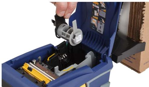
6. Pull the loose end of the bulk labels out of the box and thread over the tray and into the bulk label feed path on the printer.
