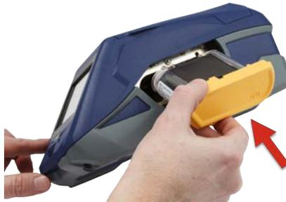
4. Turn the lock lever toward the front of the printer to lock it.
