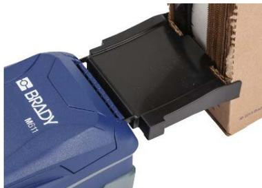
5. Insert the label spool into the printer so that the smart cell aligns with the reader in the label well. Adjust the label guide as needed.
